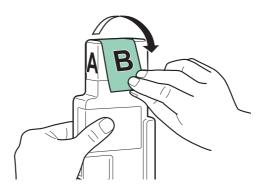
8 Seal up the old waste toner box with the supplied plastic bag and dispose of it.
